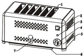
1.Bread entry slot; 2. Option switch; 3. Power indicator; 4.Timer; 5.Body of toaster; 6. Crumb tray; 7.Hi-lift toast ejector.
