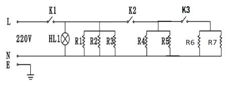
K1-timer switch K2/K3-choice Switches HL1-power indicator R1~R7-electric panels
